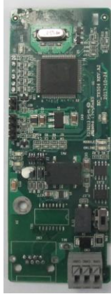
CANopen/CAN master/slave control communication card EC-TX505/511
